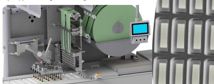
The applicator cuts efficiently multiple pads and seamlessly transfers them to the tray in a continuous motion. This process is facilitated by smoothly moving the pads from the cutting station to the tray. By changing a few size parts to make pads of a different length, accommodates the production of various tray sizes on the same production line.
