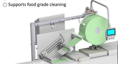
The applicator cuts efficiently one or more pads and seamlessly transfers them into the tray in a continuous motion. This process is facilitated by smoothly moving the pads from the cutting station to the tray. By changing the pad roll width and define a new length in the operators panel, the applicator accommodates the production of various tray sizes on the same production line.
